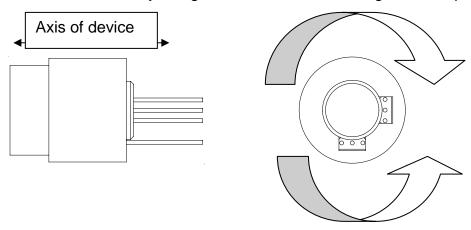
The leads can be bent to accomdidate the horizontal operation. Please note that the leads should not make contact with each other or failure of the device will occur, as with our standard devices.
