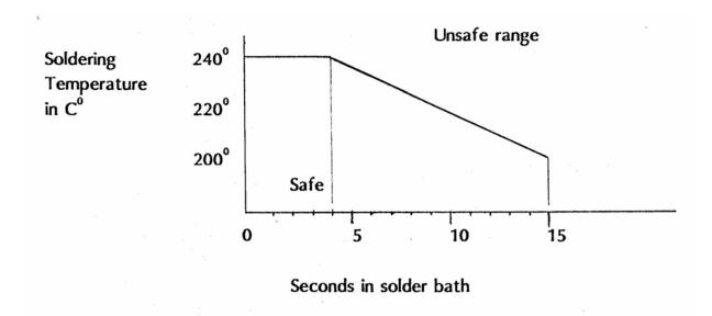
Hand soldering requires particular care for most hand soldering equipment is not accurately temperature controlled.
