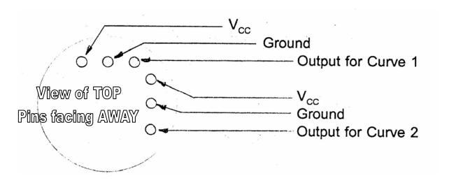
V<sub>cc</sub> should be controlled 5.00 volts. Output is ratiometric and depends on controlled input voltage. Input to sensor should be "spike" protected.
